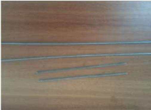
Figure 7: Photograph of the Pultruded CFRP
