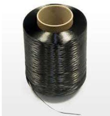
Figure 4: Carbon Fiber Reinforcement of having 9200 Tex
